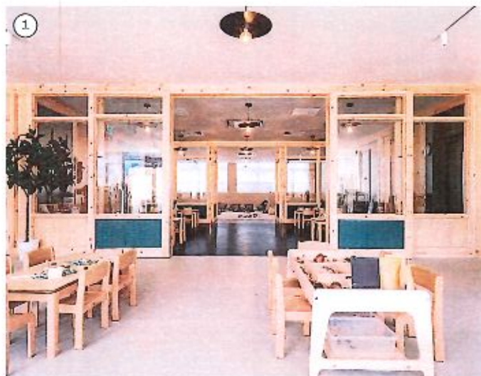
1 THE USE OF SUSTAINABLE NATURAL MATERIALS SUCH AS TIMBER, PINE-FACED PLYWOOD WALLS AND RECYCLED RUBBER FLOORING
